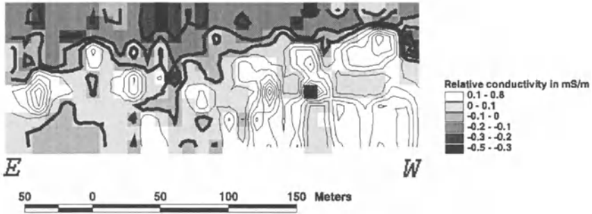
Fig. 4. Contour map of the survey area in Val Bever, Upper Engadin, Eastern Swiss Alps, with north at the bottom of the plot. The area is bounded by two forest aisles to the East and West and by a road to the North. Negative conductivity anomalies (calculated as deviations from the global mean) are shaded in grey and black and the thick black lines depict negative contours, thus bordering the areas of enhanced permafrost occurrence. The thin contours represent positive anomalies.
