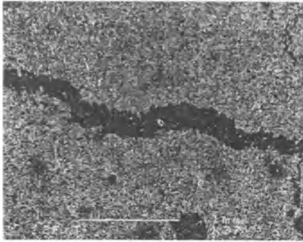
Plate 8. Scanning electron micrographs of silt and clay particles above planar pore
