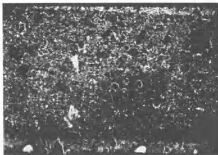
Plate 2. Microstructure of Moley Clay (unfrozen). The frame is 36 mm wide
