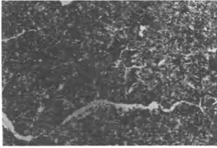
Plate 11. Fragmic morphology in Caen silt (after two freeze-thaw cycle). The frame is 12 mm wide
